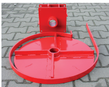
Strengthened version of the beater mill increases its service life by 3
