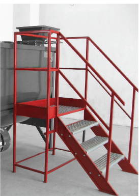
Steps with service platform
