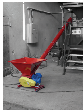
Feeding screw with charging hopper
